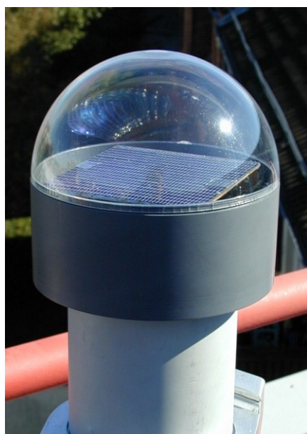
Fig. 9 Laboratory prototype of a planar antenna with solar cells for GSM 900. It is used for radio transmission and DC power supply of a wireless monitoring system (Source: ISET).
