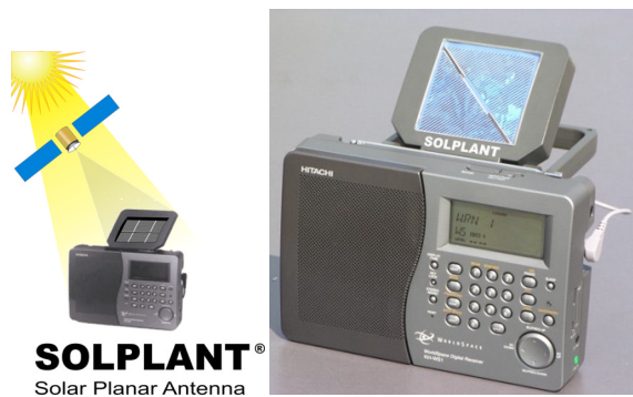
Fig. 12 SOLPLANT ® in combination with a WorldSpace Satellite Receiver for grid independent use in villages of the third world. Left: principle of simultaneous reception and PV-generation. Right: WorldSpace Receiver with a Prototype of a SOLPLANT ® Satellite Antenna (Source: ISET).
