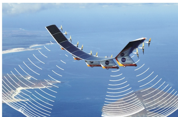
Fig. 11 Vision of the pv-powered flying wing aircraft “HELIOS”, suggested by the NASA. It is profitable to use this “atmospheric satellite” in combination with SOLPLANT ® as integrated antenna to reduce weight (Source NASA, modified by ISET).
