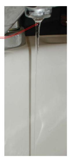
Shown above is water flowing gently from a standard bathroom faucet. The flow is just sufficient to be reasonably laminar. It is important that the flow have this closed structure, because the purpose of this experiment is to blow a bubble inside the water near the faucet. If the flow is not laminar, there is no inside to blow up.
