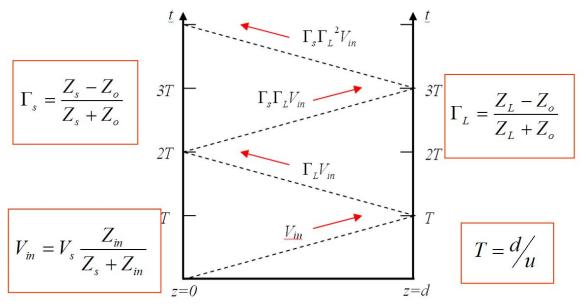
The time delay T is the measured number.
