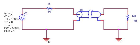
with the appropriate resistance chosen for each case. Note that there is a small delay added so that the pulses can be fully seen in the plots. Do all four cases again, using the information from the coax reel and lumped box. Here you will only need to find the voltages at the input and output ends of the cable.
