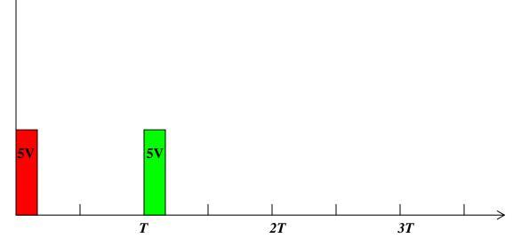
In these plots, the red pulses are at the source end and the green pulses are at the load end. The only case that requires any real analysis is #4. First pulse to the right (6.67V), first pulse reflected from the load (-2.22V), first pulse reflected from the source (.74V), second pulse reflected from the load (-.25V).
