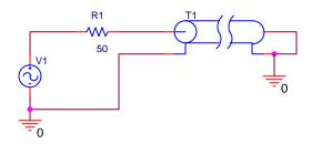
A 200 meter long air insulated transmission line has a short circuit at its load end. At low frequencies (near  $\omega=0$ ), does the line look like an inductor a capacitor or a resistor? (Circle the correct answer.) Which of the following frequencies are low? (Again, circle the correct answers.)
