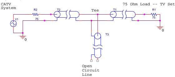
An open-circuited, 0.20 meter long transmission line with  $Z_o = 75\Omega$  and  $v_{ph} = 2.5 \times 10^8$  m/s connected to a CATV line with a Tee, as shown. Which of the following channels will be blocked by this line? (The frequencies are given in MHz.)
