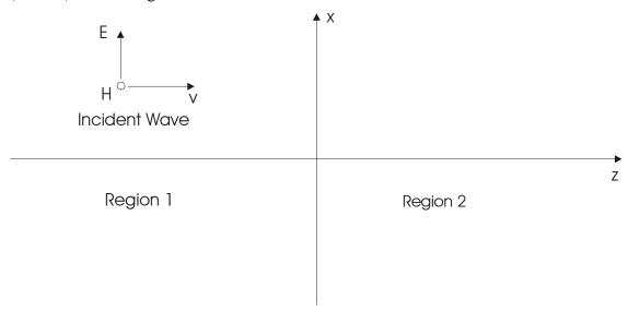
A uniform plane wave is incident normally on a dielectric interface between two media. Region 1 is air and region 2 is a dielectric region with  $\varepsilon = 4\varepsilon_o$ . The incident electric field is polarized in the x-direction and the magnetic field is polarized in the y-direction. The magnitude of the incident electric field is 100 V/m and the frequency of the wave is 10 MHz.
