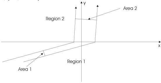
Shown above are two parallel magnetic field  $(\vec{B})$  lines changing direction at the boundary between a magnetic material (with  $\mu = \mu_r \mu_o$ ) and air  $(\mu = \mu_o)$ .
