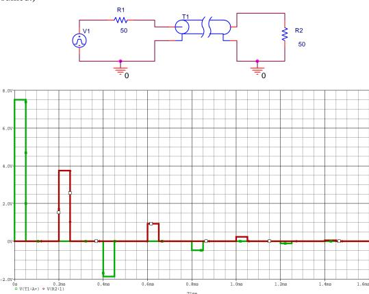
a. First, identify the input and output voltages in the diagram above. Then, determine the time it takes for the pulse to propagate from the input to the output of the transmission line. From this information, determine the relative permittivity  $\varepsilon_r$  of the insulating material used in the cable.
