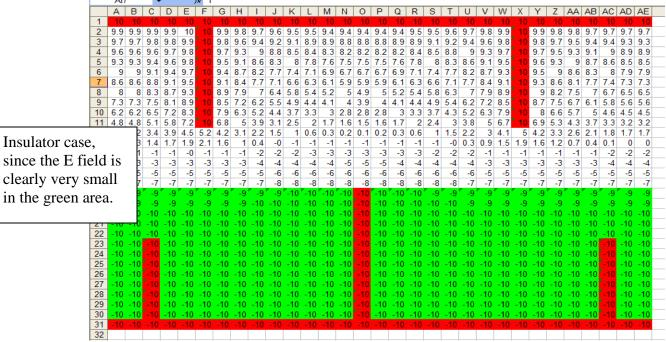
Note that the two electrodes are at voltages of +10V and -10V.
