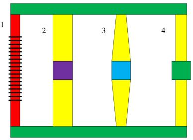
The magnetic circuit at the left consists of four legs. The leftmost leg is wrapped with N turns of wire carrying a current I. Each of the legs looks the same from each side. The square sections in the middle of the second, third, and fourth legs are identical cubes. The permeability of the cubes is  $\mu_{cube}$  and the permeability of all legs, including the horizontal legs at the top and
