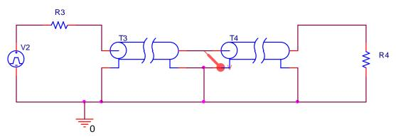
Using the same configuration as in the previous problem, a *10V*, *50ns* pulse was input to line T3 and measured at the input to T4, with the result shown below. (These are the same lines as in the previous problem, but have different names to keep PSpice happy.) Also, R3 and R4 are the same.
