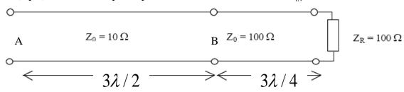
At B,  $Z_{IN} = Z_o = 100\Omega$  because the second line is matched. At A, $Z_{IN} = Z_L = 100\Omega$  because the first line is a multiple of a half wavelength.Fields and Waves IQuiz 1K. A. Connor28 September 2009
