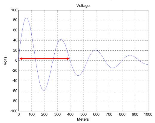
*The red line in the figure shows the distance equal to*  $1.5\lambda = 400$  *so that*  $\lambda = \frac{800}{3} = 266.7$
