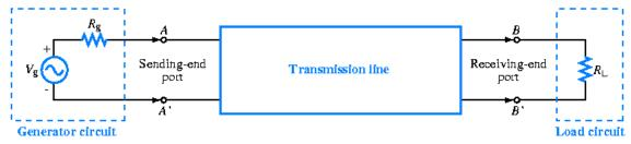
Assume a sinusoidal source is connected to a lossless transmission line, as shown.
