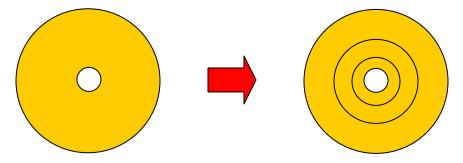
The center insulator will be chosen to have the largest breakdown voltage, the other one or two insulators will be chosen to obtain the same capacitance. Recall that each will have a different dielectric constant. To find material properties, you can go to MatWeb <a href="http://matweb.com/">http://matweb.com/</a> which has almost any property one can think of for commercially available materials.
