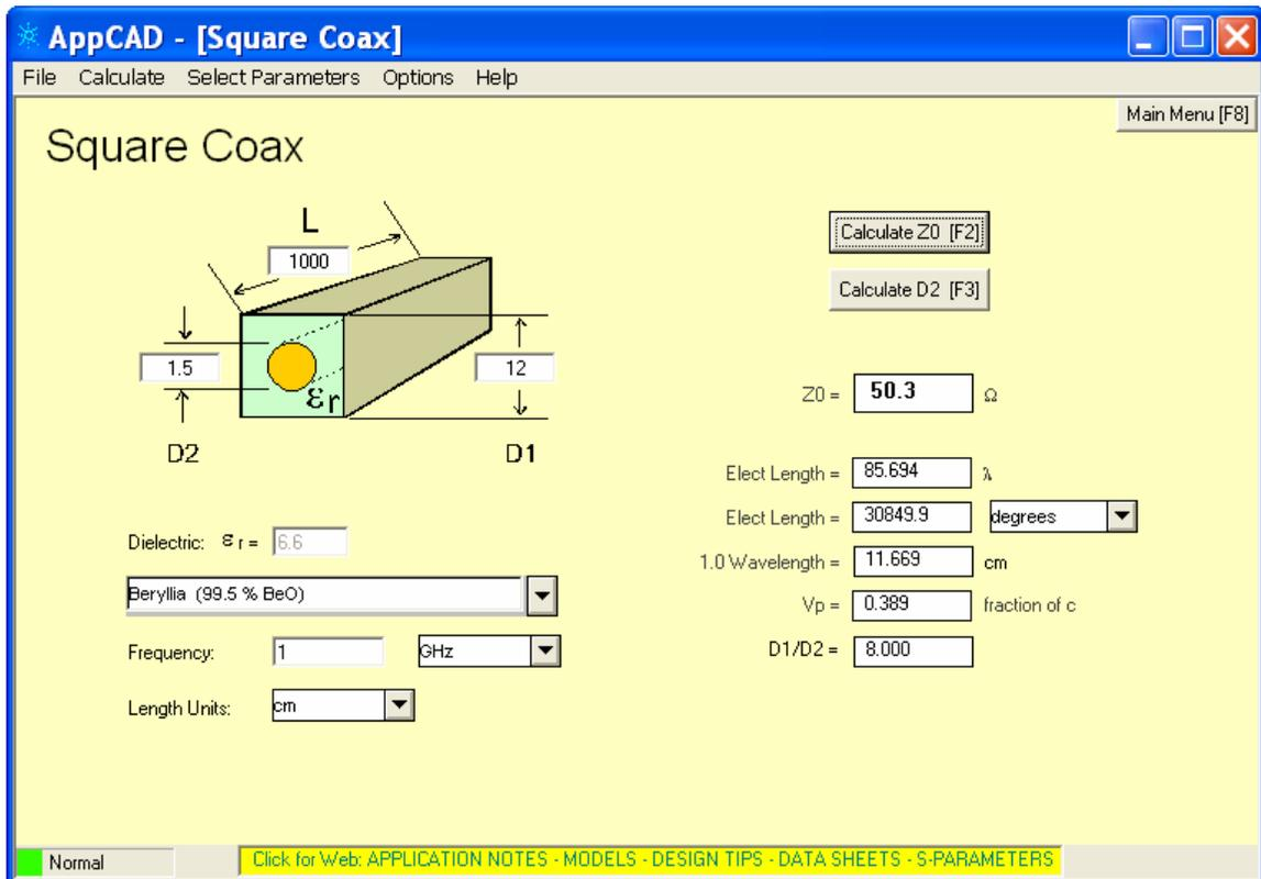
From the options available, beryllia gives the best result. With a wave propagation speed of .389 the speed of light, we can figure out the capacitance and inductance per
