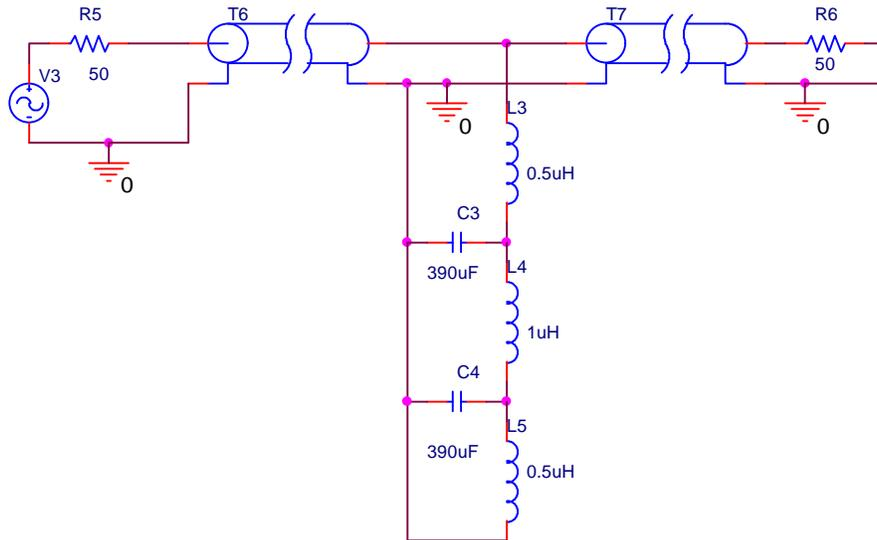
Notice that the short circuit now does not eliminate any of the components. Unfortunately, there is no good way to build a lumped model of a transmission line that works exactly right for both a short and an open circuit load. With our new model, the last inductor would be ignored if the load was an open circuit. For the new model the voltages at the input and output now look much more like the ideal line case. The voltages are still not exactly the same.
