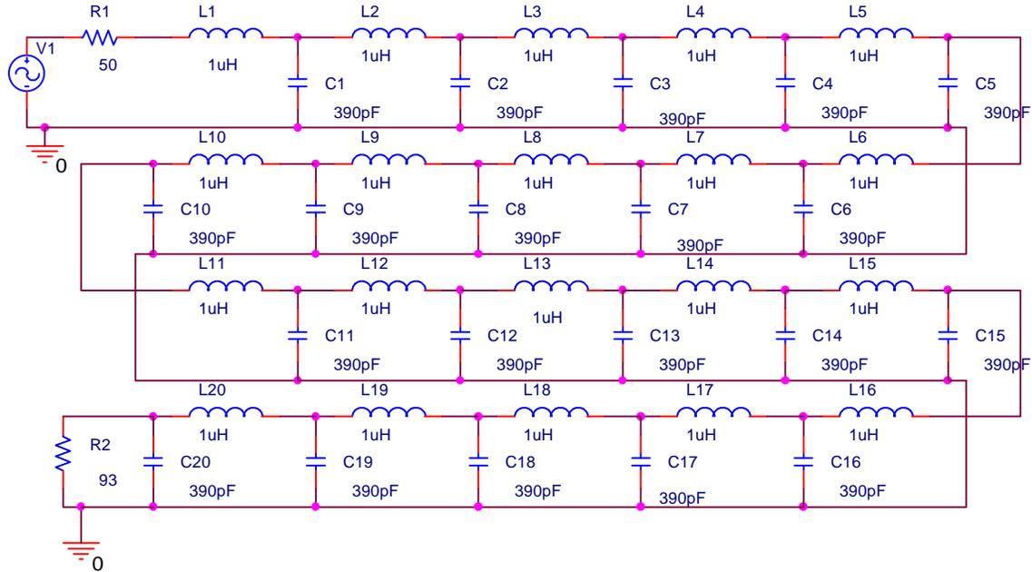
The physical circuit has one BNC connector at the input end and a BNC connector and two banana plug connector posts at the output end. This circuit can be modeled using PSpice to determine its frequency response. The input voltage as a function of frequency looks like:
