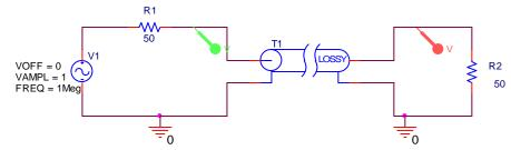
Assume we have a transmission line for which we know nothing, except its length (24 meters). We set up the standard configuration shown above and find the following voltages at the input and output ends as a function of frequency:
