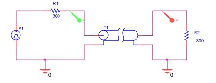
Assume that a pulsed source is matched to its line and load. That is  $R_g = R_L = Z_o = 300$ Ohms. The propagation velocity on the line is  $u = 2x10^8$  m/s. A 1 microsecond voltage pulse is launched on the line. The following voltages are observed at the input and output of the line:
