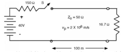
A 40V DC source with a 150 Ohm internal impedance is connected to a 50 Ohm transmission line with a 16.7 Ohm load. The length of the line is 100 meters and the propagation speed is  $2x10^8$  m/s.
