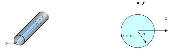
A long, straight, solid cylindrical conductor with a radius of a is shown above. The surrounding medium is free space. There is a total current  $I_o$  carried by this conductor directed **into the page**.
