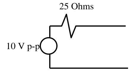
The amplitude of the forward wave down the line is found from a voltage divider rule with the line being represented by  $Z_0$ . Find the amplitude of the forward wave. For an 80 meter long cable, what is the delay time? The spools are not quite 80 meters long so find the length by looking at the transit time of the wave.
