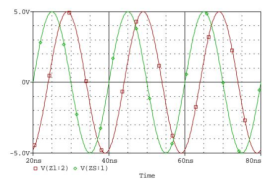
The above figure is a plot of the voltage as a function of time at the input and the output of a  $Z_0 = 300 [\Omega]$ ,  $v_p = 2.5E8 [m/s]$  transmission line. V(ZS:1) is the input voltage and V(ZI:2) is the output voltage. This plot is similar to those we made performing the experiments in Lesson 1.1, though notice that the line parameters are different. The PSpice circuit is shown on the next page.
