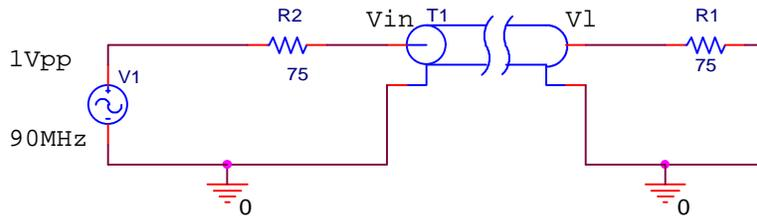
where  $R_1$  is the input to the television set and  $R_2$  is the output impedance of the amplifier. The voltage level shown is arbitrary, not realistic. The voltage at the input to the transmission line  $V_{in}$  and the voltage across the load resistor  $V_1$  look like the following:
