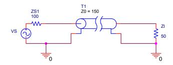
For the above circuit, determine the input impedance for the following line lengths,  $l = \frac{\lambda}{100}, \frac{\lambda}{8}, \frac{\lambda}{4}, \frac{3\lambda}{8}, \frac{\lambda}{2}, \frac{3\lambda}{4}, \lambda$ .
