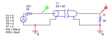
The above circuit represents a 50 [ns], 5 [V] pulse sent down a 100 [m], 50 [ $\Omega$ ], 2E8 [m/s] transmission line with matched source and load impedances.
