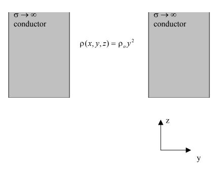
In the above figure, a charge distribution lies between two conductors. The geometry is infinite in the *z*-direction.
