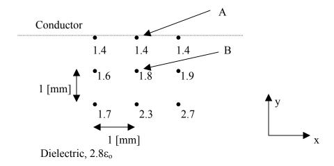
In the above figure, the voltage at each point is shown. Approximately, what is the electric field (in vector form) at points A and B?
