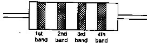
The first and second bands represent digits, while the third band indicates the power of 10 by which to multiply. The fourth band indicates the tolerance of the indicated value. A silver band represents a tolerance of 5%, and a gold band indicates 10%.
