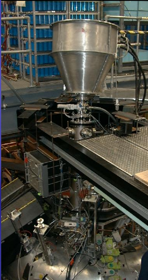
Heavy Ion Beam Probe on Madison Symmetric Torus, primary beamline
