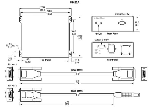
The 87422A power supply provides the dc power needed to bias the 8302A, plus an additional ±12V dc output.
