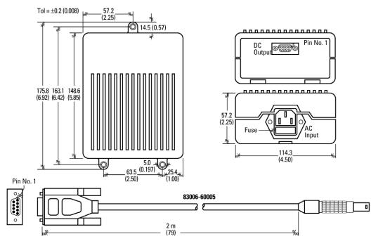
The 87421A power supply provides the dc power needed to bias the 83006A, 83017A, 83018A, 83050A, and 83051A.
