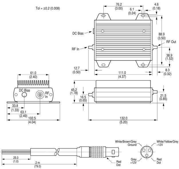
83006-60004 dc bias cable. Cable shipped with 8300A, 83017A, 83018A, 83050A, and 83051A.
