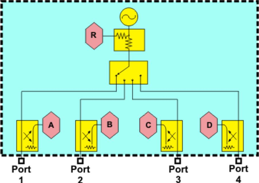
**N5230A/C Option 145 or 245 Configurable Test Set and Extended Power Range**
