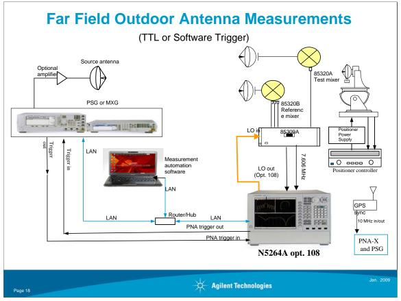
This slide is the same as few slides ago. However, I have not mention using LAN as interface instead of traditional GPIB. LAN is fast and goes longer distance when compared to GPIB.
