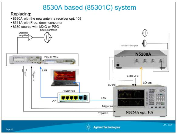
This slide shows the complete replacement. 8360 source replaced by MXG, which provides higher measurement speed. In addition, LAN is used instead of GPIB interface.
