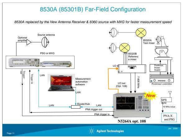
This configuration replaced 8360 sources with the MXG for transmitting side and Antenna receiver option 108 as LO source to the 85309A. This configuration provides the highest measurement speed for Far-field application, because the MXG source frequency switching time is ten times faster than 8360. Controlling external source via internal antenna receiver firmware. This is same as 8530A operation.
