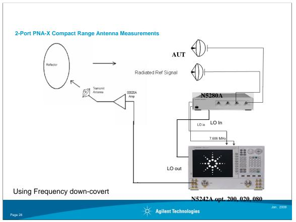
This slide shows a typical compact range using PNA-X for both transmitting source and rear LO output for LO source.
