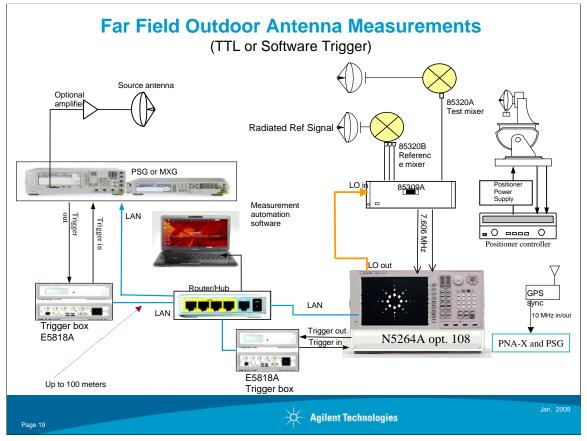
This slide shows the LAN Hub and Trigger box that extends the distance between receiving and transmitting even farther. For example, this configuration extends 100 meters on side of the LAN Hub.
