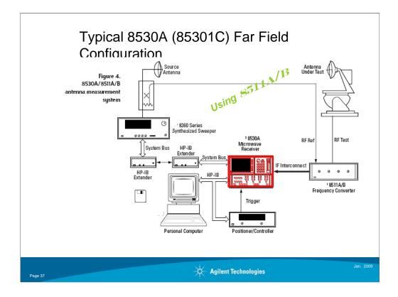
This configuration is using HPUX worstation to drive 8530A. Customer provided software in HPBASIC to control 8530A and positionner. 8360 series as RF sources driven by 8530 (system GPIB)
