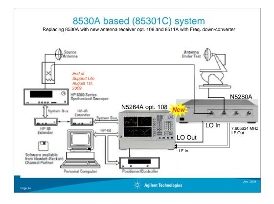
Here is new configuration with the antenna receiver option 108. 8530A replaced by new antenna receiver and the frequency down-converter, N5280A replaced 8511A. 8360 source still in placed.
