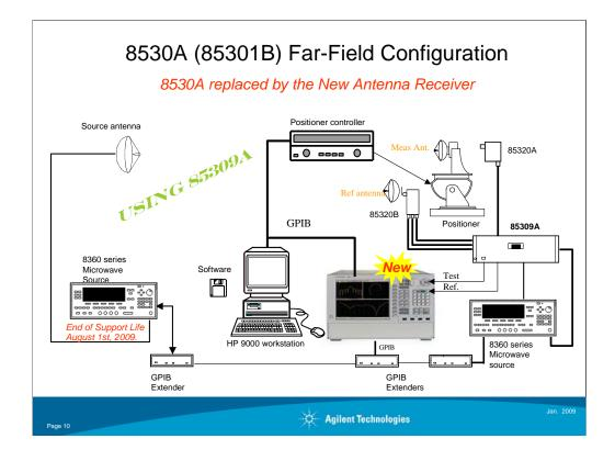
This is the same previous slide but the 8530A replaced by the new antenna receiver. All other system components stayed the same. With the 8530A code emulation, the system should just work.
