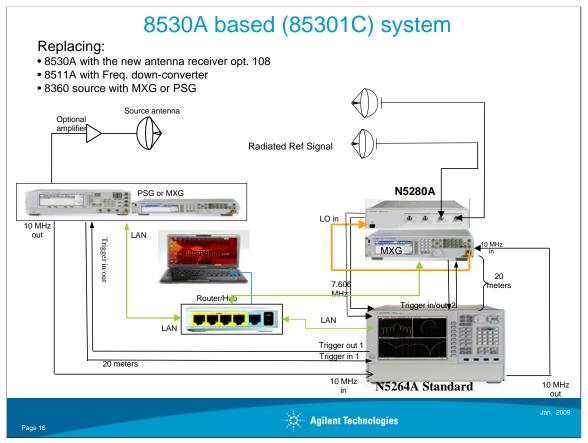
In some antenna ranges, the distance from antenna receiver and antenna itself may be too far. Some of these configurations, the external source must be used for LO input to the frequency down-converter.
