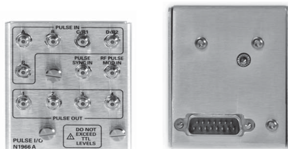
Pulse I/O adapter (N1966A) simplifies connections
