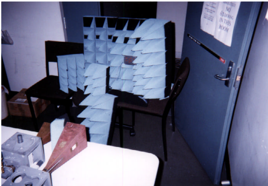
Fig 5.3. Experimental setup for quasi-optical amplifier gain measurement
