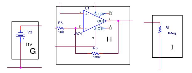
a. Identify the function of each of the nine blocks. (Draw a line to connect the letter of the block to its function). (9 points)
