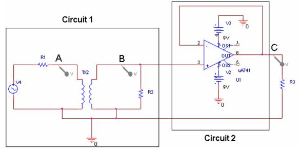
a) What is circuit 2 called and what does it do? (3 points) Circuit 2 is a voltage follower (or buffer). It isolates the input from the output so the circuits on either side do not influence each other.
