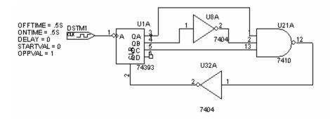
Here is the output from PSpice. You can see that it counts to four before the reset spike (U1A:CLR) resets it. (Observe that the reset actually comes when the counter outputs a five.)
