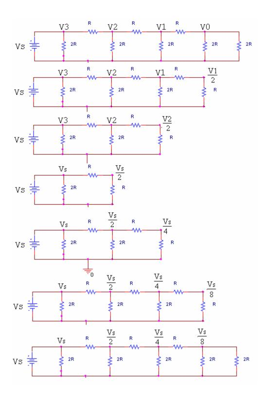
b) If we assume that closing switches has negligible effect on the voltage levels we found in part a), what will be the output of the DAC circuit, Vout (in terms of Vs), when the input (b3 b2 b1 b0) is: (10 points)
