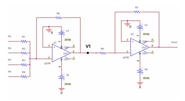
a) Select values for R1, R2, R3, and R4 so that the output voltage will be the decimal equivalent of DCBA. For example, if DCBA=1010, or equivalently VD=VB=5 V, VA=VC=0 V, then Vout = 10 V. The circuit should work for <u>all</u> possible DCBA combinations. (*12 points*)
