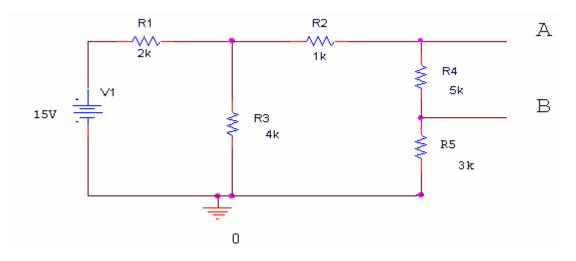
a) (6 points) Find the Thevenin voltage (Voc) of the circuit assuming the load will be connected between A and B.
