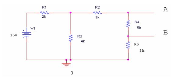
a) (6 points) Find the Thevenin voltage (Vth) of the circuit assuming the load will be connected between A and B.
