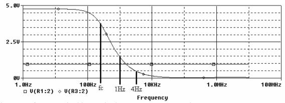
The corner frequency in this case is about 200 Hertz. Note that answers may vary. Corner frequencies should be at or below 500Hz.
