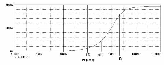
The corner frequency in this case is about 20K Hertz. Note that answers may vary. Corner frequencies should be at or above 8K Hz
