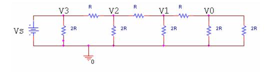
b) If we assume that closing switches has negligible effect on the voltage levels we found in part a), what will be the output of the DAC circuit, Vout (in terms of Vs), when the input (b3 b2 b1 b0) is: (*10 points*)
