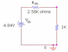
d) (4 points) Find the voltage between A and B for this circuit with a load of 1K ohms. VAB = (Vthx1K)/(1K+Rth) = (4.84x1k)/(1K+2.58K) = 1.35 voltsVAB = 1.35 volts
