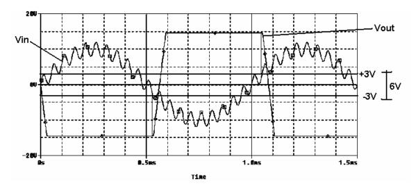
b) Estimate the value of the hysteresis for the Schmitt trigger model AND indicate the hysteresis range on the output plot. (8 pts).
