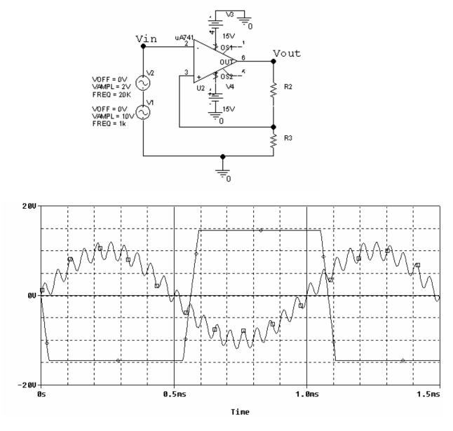
a) Indicate Vin and Vout for the model of a Schmitt trigger above on the output plot below (4 pts).
