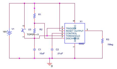
The circuit above has been simulated using PSpice. Using PROBE, the voltages at pins 2, 6, 7, and 3 have been displayed.
