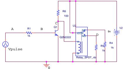
In the circuit above, the voltage source Vpulse puts out a sequence of pulses and the voltages at the source and three other points are monitored (marked A, B, C and D). You will note that this circuit is like the one we used in Exp 10 and in the Clapper project. The relay model used by PSpice (which gives switch times, circuit parameters, etc.) is listed below:
