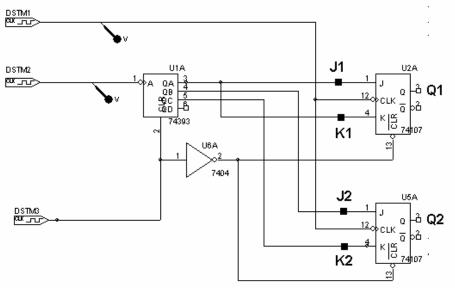
a) Complete the timing diagram for the circuit above. Note that the first trace shown is DSTM1 (flip flop clock), the second trace shown is DSTM2 (counter clock), and DSTM3 provides an initial reset pulse to both of the devices. You can assume that all outputs are initially 0 and that all three devices change on the falling edge of the clock. Draw traces for all six of the points indicated: (J1, K1, Q1, J2, K2, Q2) (*3 points each* = 18 points)
