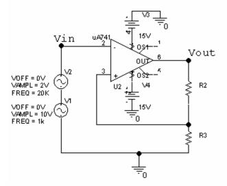
a) Indicate Vin and Vout for the model of a Schmitt trigger above on the output plot below (4 pts).
