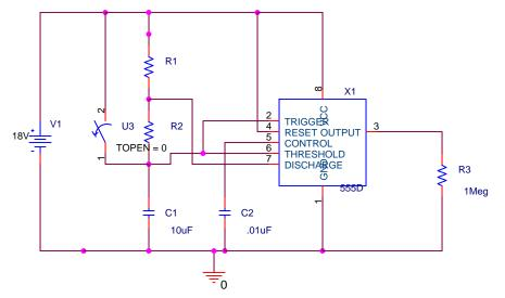
The circuit above has been simulated using PSpice. Using PROBE, the voltages at pins 2, 6, 7, and 3 have been displayed.
