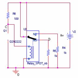
$$\label{eq:VD} \begin{split} VD &= 9V \\ VC &= V2*R_{relay}/(R_{relay}+R6) = 9(100)/(100+100) = 4.5V \end{split}$$
