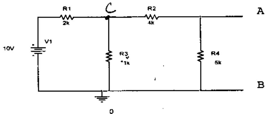
a) Find the Thevenin Voltage ( $V_{oc}$ ) of the Circuit (8 points)
