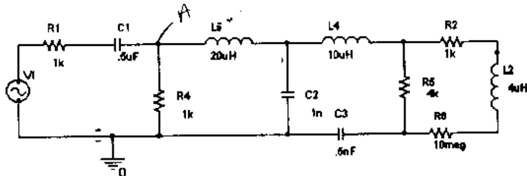
Given that you know that inductors and capacitors can behave like short and open circuits at very high and low frequencies, we want to redraw the above circuit by replacing components that look like open circuits by open circuits and components that look like short circuits by short circuits.
