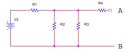
Let V2=12V, R1=50 ohms, R2=1K ohms, R3=2K ohms, and R4=500 ohms.
