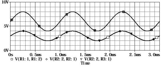
The plot below is correct. The DC voltage is 6V for R1 (square), and 3V for R2 and R3 (triangle and diamond). The amplitude across R1 is about 0.8V and over R2 and R3 is half that. The voltage across R2 and R3 must be the same because they are in parallel.
