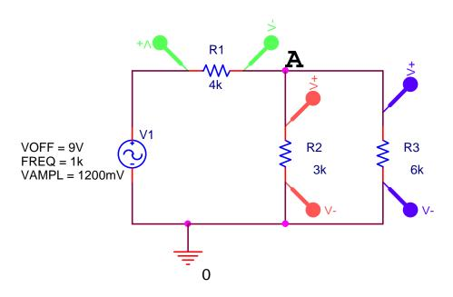
a) Given the circuit above, calculate the DC offset voltage at point A. (5 points)
