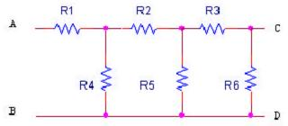
The total resistance between A and B is R1 + R4 // [R2 + R5 // (R6+R3)]Test A: R63 = 2K+2K=4K R563=2K\*4K/(2K+4K)=1.33K R2563=2K+1.33K=3.33KR42563 = 2K\*3.33K/(2K+3.33K)=1.25K R142563=2K+1.25K = 3.25K ohms
