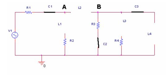
2) What is the amplitude of the voltage at point A at high frequencies? (2 points)
