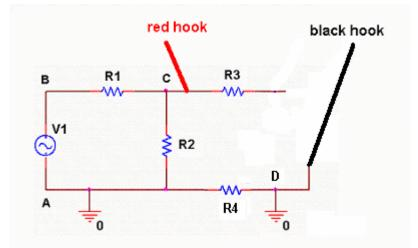
R4 is grounded on both sides, so it is not part of circuit. R3 has no current flowing through it, so it is also not part of the circuit. This is just a voltage divider using R1 and R2. R1=3.9KR2=16k
