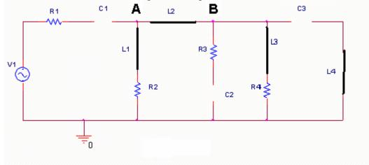
2) What is the amplitude of the voltage at point A at low frequencies? (2 points)
