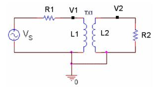
In the transformer circuit above, R1 = 400 ohms, R2 = 20K ohms, and the turns ratio of the transformer is 1:5. Assume the transformer has perfect coupling. [Hint: You cannot assume that R1 is much smaller than R2.]
