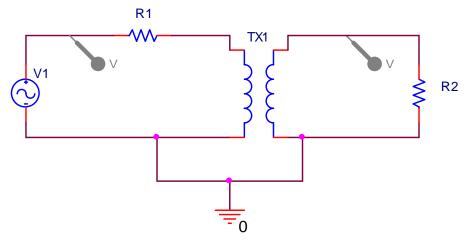
$$L1 = 1 \text{mH}, k=1, R1 = 5\Omega, R2 = 5 \text{K}\Omega, V1 = 200 \text{mV}$$
