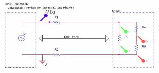
V1: VOFF=3V VAMPL = 5V FREQ = 1KHz R1=27.3 $\Omega$  R2=27.3 $\Omega$  R3=1K $\Omega$  R4=800 $\Omega$  R5=400 $\Omega$
