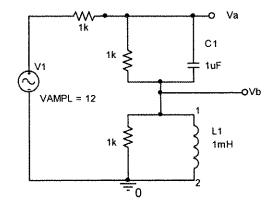
1) Redraw the circuit above for very high frequencies. Label points Va and Vb on your diagram, and be sure to include the source V1. (3 pts)
