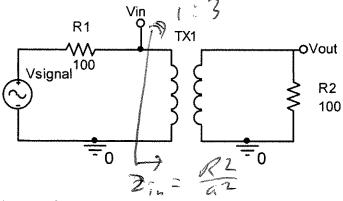
3) Assume the transformer in the circuit above is ideal with a turns ratio of 3:1. If Vsignal has an amplitude of 12V, what is the amplitude of Vin and Vout? Show your work for partial credit. (6 pts)
