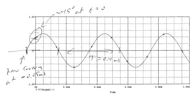
1) The voltage trace shown above is a signal measured in a circuit. Using the SIN convention, any voltage in a linear circuit can be represented by the form:  $v_x(t) = V_x \sin(\omega t + \phi_x)$
