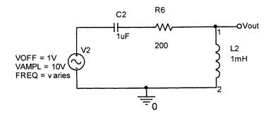
6) Redraw the circuit above for very low frequency. Label the point Vout and be sure to include V2. What is the value amplitude of Vout at very low frequencies? (3 pts)
