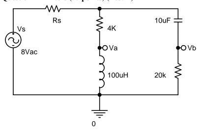
Part 1: Filters, Using Rs= $0\Omega$
