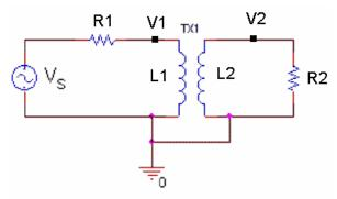
You are given the above transformer. You can assume the transformer is ideal, the coupling coefficient is 1, and the resistance of R1 is negligible compared to the resistance of R2. The plot below shows the input to the transformer at V1 and the output at V2. The output is the signal with the larger amplitude.
