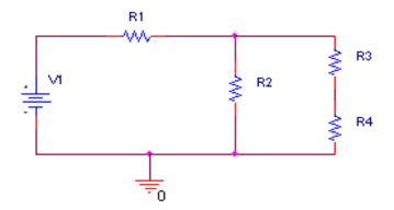
Given: V1 = 10volts, R1 = 2000Ω, R2 = 1000Ω, R3 = 1200Ω, R4 = 1800Ω.
