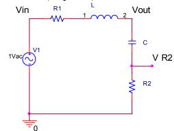
1) What is the transfer function (Vout/Vin) for the circuit in terms of R1, R2, L, & C? You must simplify. (6 pts)
