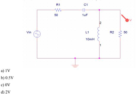
3) Given the circuit in 2), which is the most likely voltage measured across resistor R2 if Vin =  $1 \text{V} \cos(2\pi \text{ft})$ , with  $\mathbf{f} = 100 \text{kHz}$ ? (Please circle one.) (4 pts)
