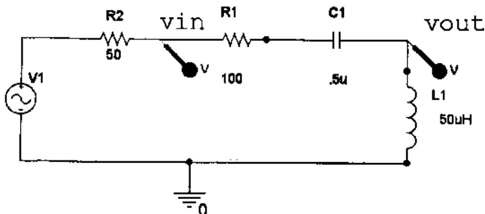
If  $v_{in}$  is the sinusoidal source (including the 50 ohm internal impedance) and  $v_{out}$  is the voltage across the inductor, is this configuration a high pass filter, a low pass filter, a band pass filter or a band reject filter? Explain your answer.
