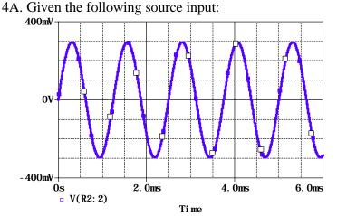
Write the mathematical expression for Vin in the form: Vin=Asin( $\omega$ t) (4 points) A=300mV T=2.5ms/2cylces=1.25ms f=800 Hz w=2pf=1.6Kp rad/sec=5.03Krad/sv(t) = 300mV sin(5.03K t)
