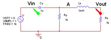
Assuming the presence of the buffer, we can assume that the output of one part of the circuit (y) is the input to the other (x). Hence:
