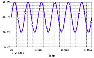
Write the mathematical expression for Vin in the form:  $Vin=Asin(\omega t)$  (4 points) A=500mV T=1us/2cylces=0.5us f=2Meg Hz w=2pf=4Meg p rad/sec=12.6Meg rad/sv(t) = 500mV sin(12.6Meg t)
