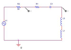
In the circuit above, V1 is a sinusoidal source and R2 is the 50 mohm impedance of the function generator. The remaining four components define some type of filter.
