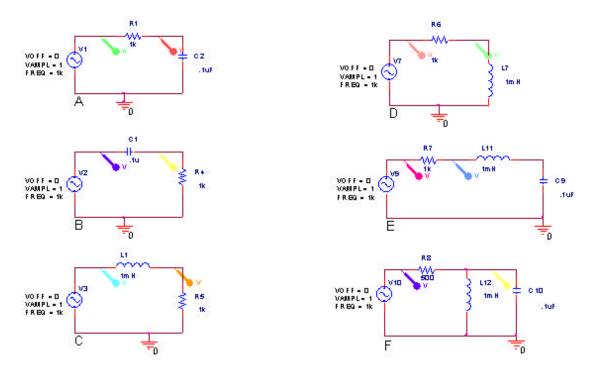
a) First, identify which type of filter these are: (6 points)Which is a low pass filter (list all): *A*, *C*
