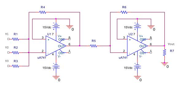
Component values for the circuit shown are as follows: R4 = 5k, R5 = 20k, R6 = 10k, R7 = 10Meg ohms. Values R1, R2, and R3 will be determined by you in part b of this question.
