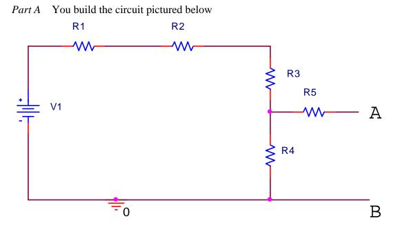
Given: R1=30 ohms, R2=2K ohms, R3 = 3K ohms, R4=2K ohms and R5=1K ohms. Given: V1=6V
