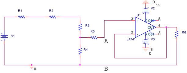
Given: R1=30 ohms, R2=2K ohms, R3 = 3K ohms, R4=2K ohms and R5=1K ohms. Given: V1=6V Given: R6 is the load of 2K ohms
