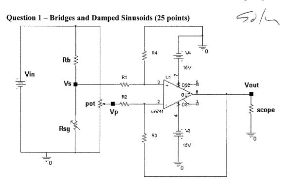
Above is figure of an amplified strain gauge bridge similar to the one you are using for project 2. The circuit has the following values: Vin = 5V, Rb=1K ohms, R1 = 2K ohms, R2 = 2K ohms, R3=10k ohms, R4=10k ohms, and the pot is a 2k pot.
