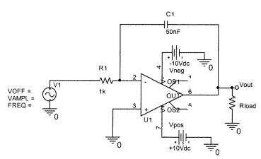
c) The circuit above is the same circuit as the one used for parts 1 and 2, but now assume that the input is sinusoidal and that we are interested in steady state response. What is  $H(j\omega)$ , the transfer function for this circuit?  $H(j\omega) = Vout/V1$ . You must use the component values, don't leave the answer in terms of R1 or C1. Simplify your answer.
