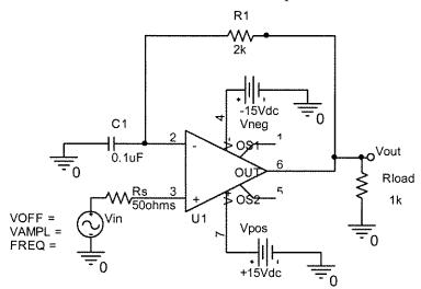
d) For this circuit, the input is sinusoidal. What is  $H(j\omega)$ , the transfer function for this circuit?  $H(j\omega) = Vout/V1$ . You must use the component values, don't leave the answer in terms of R1 or C1. Simplify your answer.
