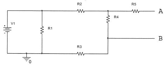
V1=6V, R1=2k ohms, R2=500 ohms, R3=1k ohms, R4=2k ohms, R5=3k ohms
