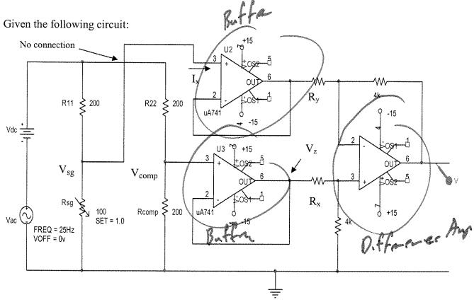
Note: Rsg is variable resistor to model a strain gauge. The SET=1.0 simple means that the nominal resistance is the full  $100\Omega$ . Use  $100\Omega$  for you analysis.
