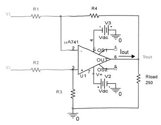
You are to use the above circuit to amplify the difference between two inputs. Assume the op-amp is ideal.
