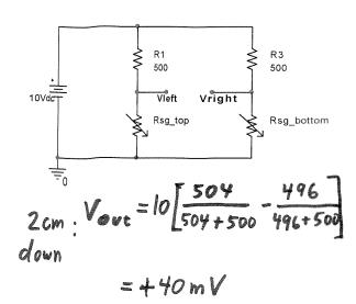
c) (1pt) Which circuit's output voltage  $v_{out}$  is more sensitive to strain gage resistance change for the same displacement?
