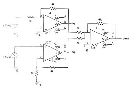
Assume that power supplies have been properly connected to all three op-amps in the circuit above. V1 is a dc source with a value of 1.5 Volts, V1(t) = 1.5 Volts. (equ. 1) V2 is an ac source which can be represented as:  $V2(t) = 0.5 \sin(2\pi 2000t) \text{ Volts}$ . (equ. 2)
