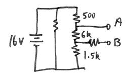
1) (5pt) Find the Thevenin equivalent voltage with respect to A and B for the circuit shown above.
