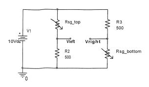
a) (4pt) If the beam is pulled up 1cm, the resistance of the top strain gauge decreases by  $2\Omega$ , and the resistance of the bottom stain gauge increases by the same amount. Fill in the table below:
