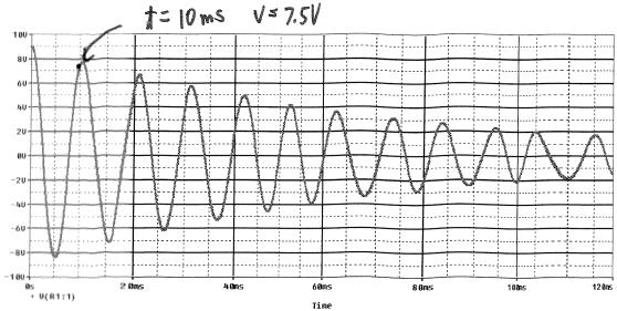
1) The figure above is the output signal from an amplified strain gauge bridge similar to the one you are using for experiment 5. The signal has the form of:  $v(t) = V_0 e^{-\alpha t} \cos(\omega t)$  and has been calibrated to indicate the displacement of the end of the beam as a function of time. The initial voltage at t = 0 corresponds to a positive displacement of 1.8cm.
