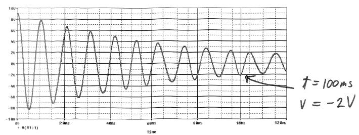
1) The figure above is the output signal from an amplified strain gauge bridge similar to the one you are using for experiment 5. The signal has the form of:  $v(t) = V_0 e^{-\alpha t} \cos(\omega t)$  and has been calibrated to indicate the displacement of the end of the beam as a function of time. The initial voltage at t = 0 corresponds to a positive displacement of 1.8cm.
