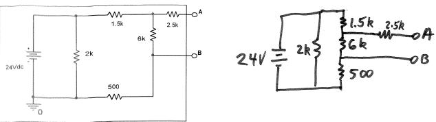
1) (5pt) Find the Thevenin equivalent voltage with respect to A and B for the circuit shown above.
