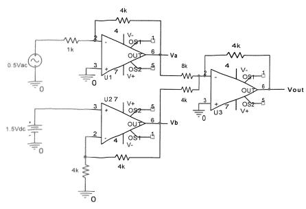
Assume that power supplies have been properly connected to all three op-amps in the circuit above. VI is an ac source which can be represented as:  $VI(t) = 0.5sin(2\pi 2000t)$  Volts. (equ. 1) V2 is a dc source with a value of 1.5 Volts, V2(t) = 1.5 Volts. (equ. 2)
