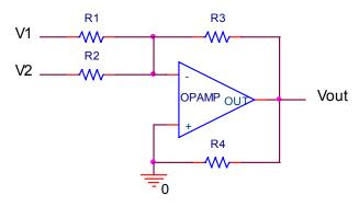
Assume that ±9 Volt power supplies have been properly connected to the op-amp in the circuit above.
