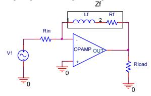
1) (4pt) Find the transfer function  $H(j\omega) = Vout(j\omega)/V1(j\omega)$  for this circuit. (Substitute in the values provided for the components.)
