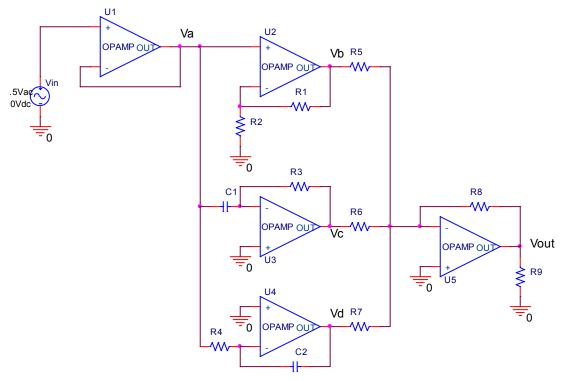
Assume that  $\pm 9$  Volt power supplies have been properly connected to all five op-amps in the circuit above.
