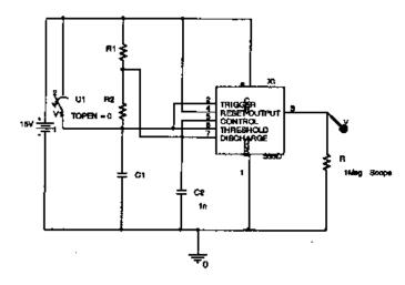
a) Design an astable multivibrator, as shown above, using R1, R2, and C1. The output should have a frequency of 5000 Hz, and a duty cycle of 60%. Show all work. (NOTE: It may be nessessary to carry out calculations to the hundredths or thousandths decimal to be accurate) (15 nts)
