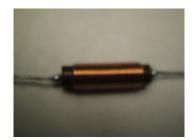
You find that it has a wire gauge diameter of 0.51 mm (24 gauge), a length of 14.5 mm, a core diameter of 5.0 mm and 27 turns. You assume that it has an air core ( $\mu = 1.257 \text{ x}$   $10^{-6}$  Henries/meter).
