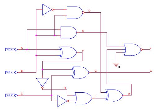
A. From the truth table for all marked points in the above circuit. (2 points each column D-K = 16 points)
