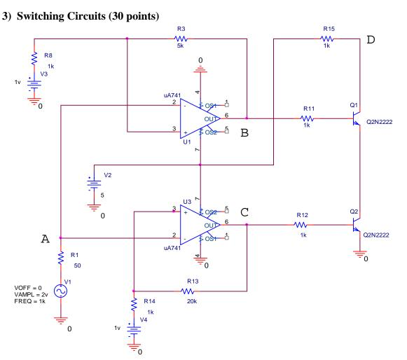
The circuit above consists of two Schmitt triggers with the same sinusoidal input signal (point A). The output of each Schmitt trigger becomes the base signal to a transistor (points B and C). The final output of the circuit is read at point D.
