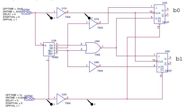
In the circuit pictured above, clock DSTM1 provides a clock signal to a counter and two flip flops. The flip flops are clocked one half cycle after the counter to allow for the propagation of the signals through the gates. (DSTM2 provides an initial reset pulse to both chips. This is required by PSpice to ensure that all sequential devices start in a known state.)
