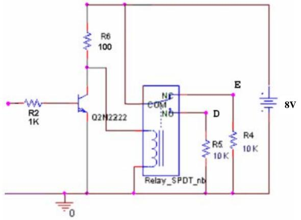
5V = 101 Output at J is low. Transistor is open. Inductor is on. VD is 8V VE is 0V R4: VE = 0V I4 = 0/10k I4 = 0 mA
