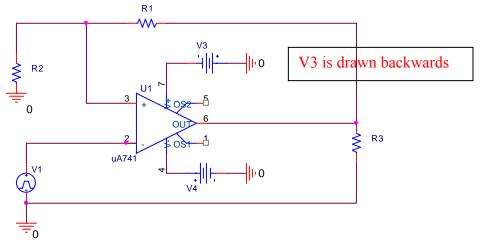
Part A: In the Schmitt trigger pictured above,  $R1 = 8k\Omega$ ,  $R2 = 1k\Omega$ ,  $R3 = 1k\Omega$ , V3 = +6V, V4 = -7V, and the input, V1, is pictured below.
