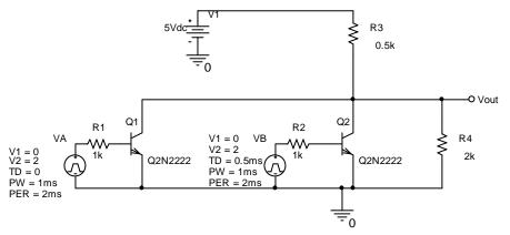
a) Redraw this circuit using the diode switch model for both Q1 and Q2. (3pts)
