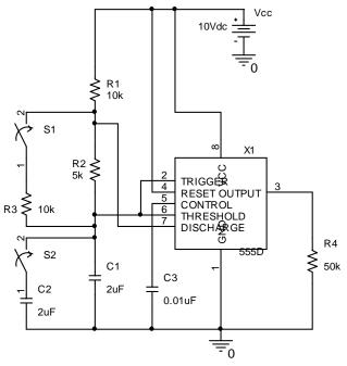
d) Using the circuit above, determine the output period and the off time with both switches open. Include units.(3pts)
