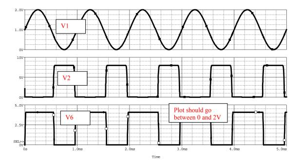
ERRORs on exam – R4 should be 50k, not 1k. Waveform on bottom plot should transition between 0 and 2V, not 0 and 4V.
