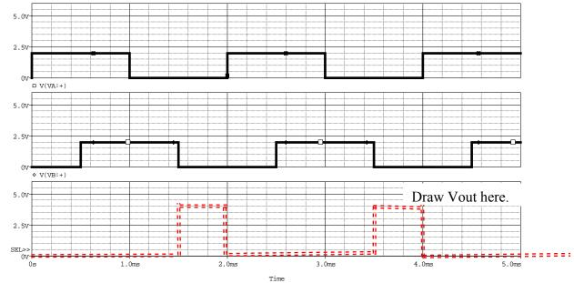
c) If VA and VB are considered to be logic inputs, and Vout is a logic gate output, then what type of gate is this? (circle one) (2pts)
