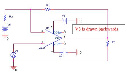
Part B: In the Schmitt trigger pictured above,  $R1 = 8k\Omega$ ,  $R2 = 1k\Omega$ ,  $R3 = 1k\Omega$ , V3 = +6V, V4 = -7V, V5 = 2V and the input, V1, is pictured below.
