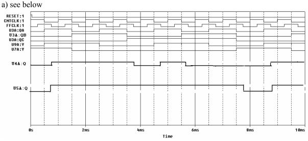
b) b0=U4A :Y=0 b1=U4a :Y=1 b2=U3A:QC=1 Binary = 110 Decimal = 6 c) Sequential logic devices have a clock that controls the timing, whereas combinational logic gates do not.
