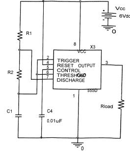
2. (5pt) Sketch the voltage waveform on pin 2 (which is tied to pin 6). Note the scales on the x and y axes. Start the plot at the time when C1 is charged to its maximum voltage.
