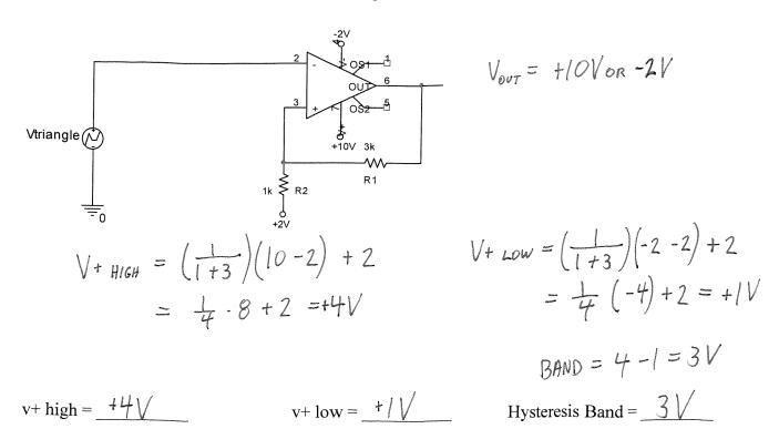
4. (3pt) If the input triangle wave to the circuit in 3. has an amplitude of 5Vp-p, what offset must be added to it to obtain a square wave on pin 6 with a 50% duty cycle that switches between -2V and  $\pm 10\text{V}$ ?
