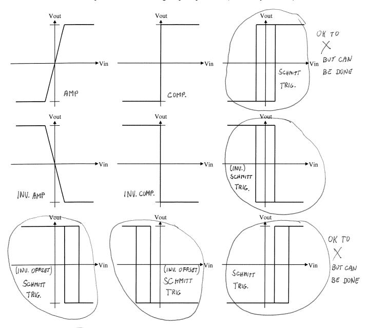
2. (2pt) TRUE or FALSE (circle one) Schmitt Triggers that include an offset reference voltage always have the reference voltage in the center of the hysteresis band.
