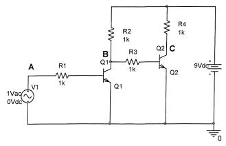
1. (6pt) For the switching transistor circuit above, fill in the voltages in the table.
