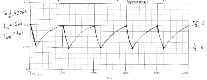
3. (4pt) If the values of C1 and Vcc double, what are the new frequency and duty cycle of the output waveform on pin 3?  $V_{cc}$  HAS NO EFFECT ON f OR DVTY CYCLE
