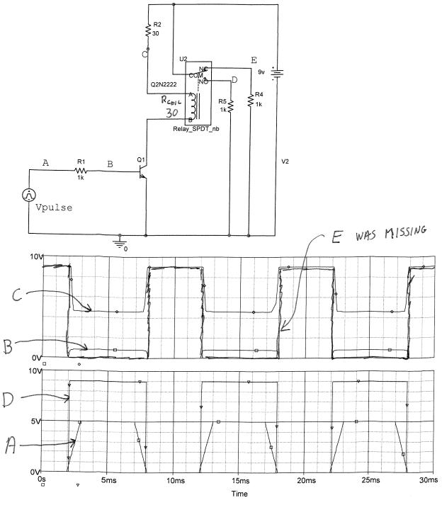
5. (3pt) If the relay coil can pass a maximum of 200mA, what is the smallest value R2 can have?
