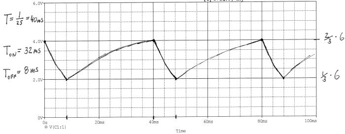
3. (4pt) If the value of C1 is halved and Vcc doubled, what are the new frequency and duty cycle of the output waveform on pin 3?
