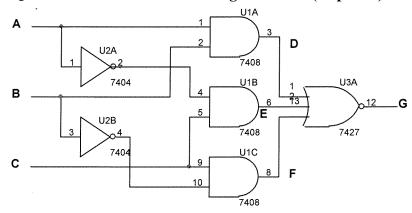
1. (6pt) Fill in columns D – G in the table below for the circuit above.
