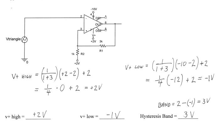
4. (3pt) If the input triangle wave to the circuit in 3. has an amplitude of 5Vp-p, what offset must be added to it to obtain a square wave on pin 6 with a 50% duty cycle that switches between -10V and +2V?
