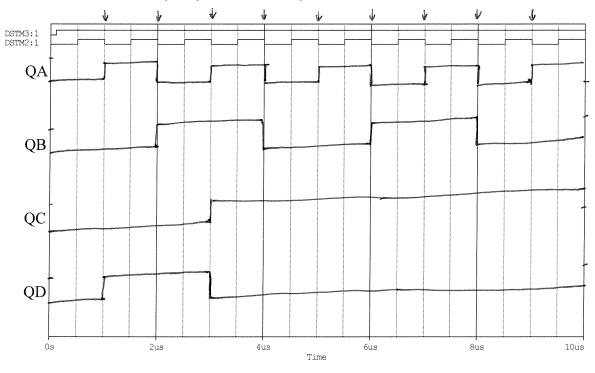
2. (2pt) How would the Q outputs in 1. change if the reset pulse remained low for the duration (10us)?
