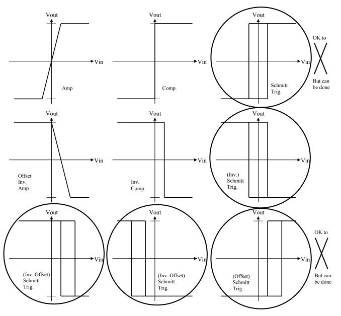
2. (2pt) TRUE or FALSE: (circle one) Schmitt Triggers that include an offset reference voltage can have a high threshold voltage > 0V while the low threshold voltage < 0V.
