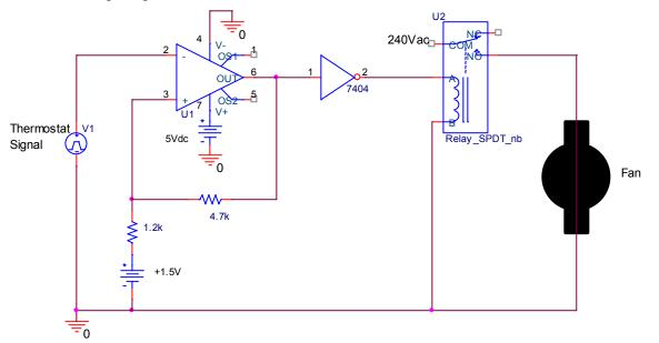
1. (6pt) For the above circuit, find the two Schmitt trigger switching voltages.
