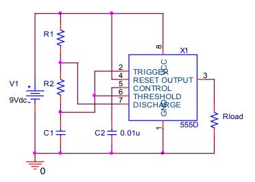
2. (4pt) Using a ratio of R1/R2 = 3 and with  $C1 = 30\mu$ F, calculate the values for R1 and R2 needed to yield a frequency of 10Hz.
