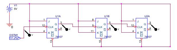
In the circuit pictured above, clock DSTM1 provides a clock signal to the first JK flip flop. This circuit follows the falling edge of the clock.
