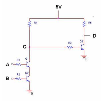
a) Redraw the figure above with the transistors modeled as a switch and a diode. (7 *points*)
