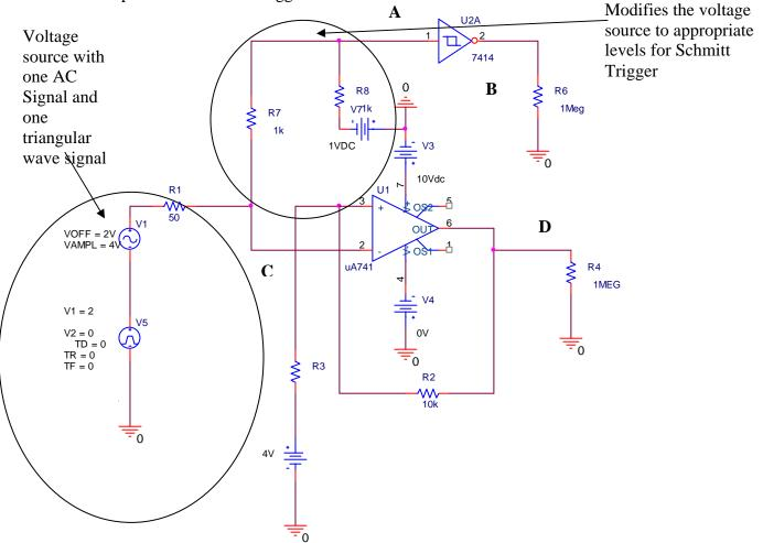
The voltage source is a combination of two sources – one is sinusoidal and one is a triangular wave The latter source has the higher frequency. The voltage levels for the op-amp Schmitt Trigger circuit are higher than for the commercial Schmitt Trigger. Thus, two resistors and a voltage source are used to change the input voltages to levels appropriate for a logic circuit. Note that we are also operating the op-amp in an unbalanced mode with the negative voltage source set to zero.
