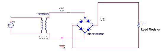
5. (7pt) Now a full wave diode bridge replaces the diode. For this question, assume that the voltage at V2 is a 12V sine wave with no offset and a frequency of 500Hz. Plot V2 and the voltage across the resistor R1.
